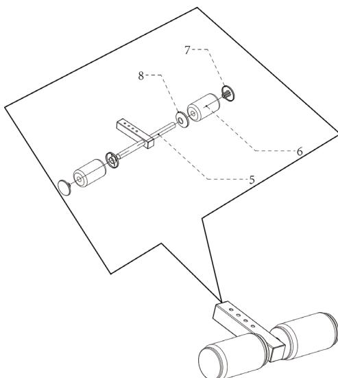
Put the covers (8) and the sponges (6) on the leg handle crossbars (5). Then put the plugs (7) on, as shown on the picture.
