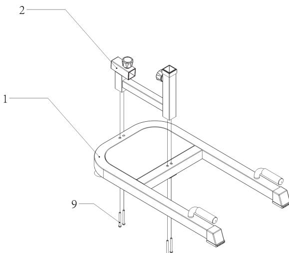
Screw the bracket base and leg handle base (2) to the main frame (1) with the screws (9). Screw them tightly with hex key (10).
