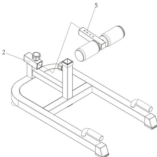
Put the leg handles (5) in the frontal bracket base profile and leg handles (2), then tighten it with the knob.
